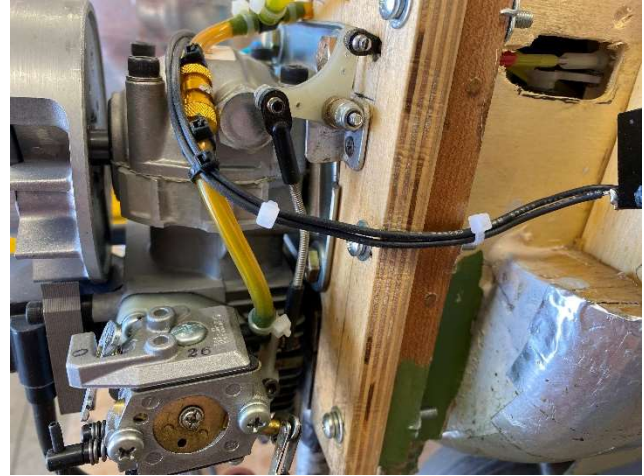
This shows the carburetor and its control linkage.
