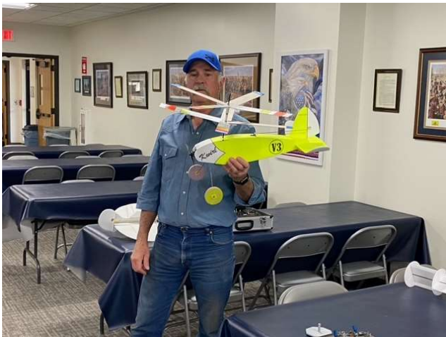
This is a gyrocopter and the blades turn in opposite directions.
