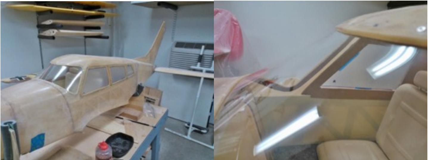
The windows are attached to a window frame then bolted to the body with 1-72 bolts. This is very much like the full size plane. You can also see the interior is installed for final testing for fit.
